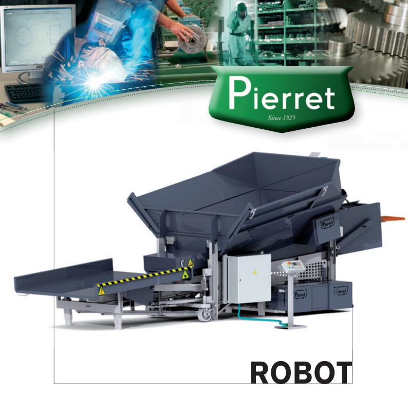
The patented "ROBOT" loader-feeder is designed to take large bales and/or boxes as well as material in bulk form and feed the material to awaiting downstream equipment such as a cutting machine. Its operation is fully automatic, consistent, adjustable and continuous. Processed material may consist of fibers, tangled yarns, rags, carpets, plastic films, tows, non-wovens, ...
